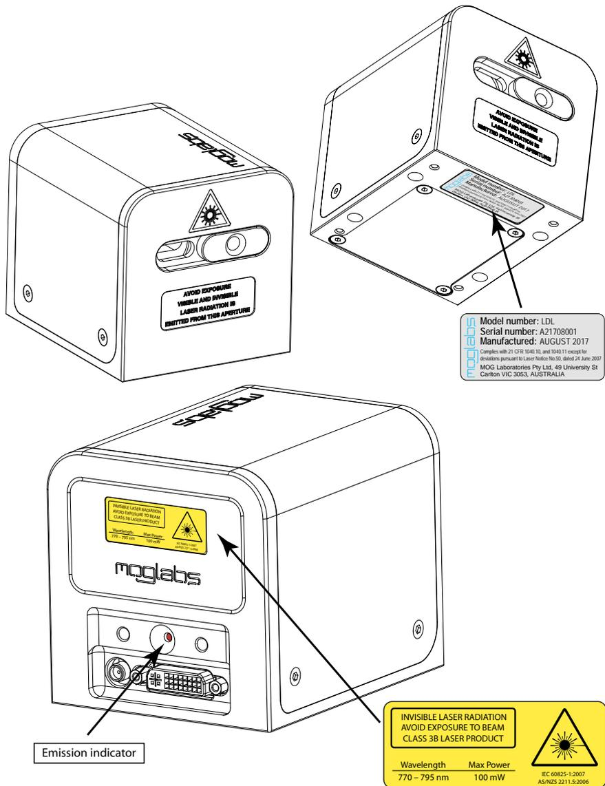
**Figure 2:** Schematic showing location of laser warning labels compliant with International Electrotechnical Commission standard IEC 60825-1:2007, and US FDA compliance label. Aperture label engraved on the front of the laser near the exit aperture; warning advisory label on the rear and compliance label beneath.
