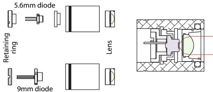
**Figure 4.1:** Lens tube assembly, showing diode, lens, and mounting hardware. The same tube can be used for 5.6 mm and 9 mm diodes.
