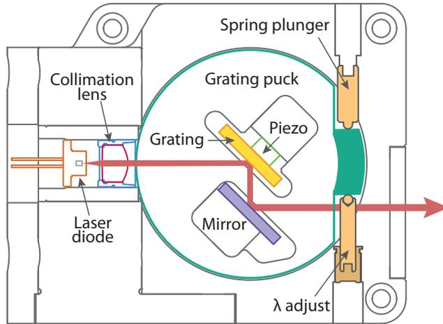
**Figure 3.1:** Cross-section sketch of the MOGLabs LDL, showing the cylindrical grating mount (puck), piezo-mounted grating, fold mirror, and wavelength adjustment. The grating mount can be rotated using the tangential  $\lambda$  fine adjustment screw. A counteracting spring-plunger should be released to allow rotation.
