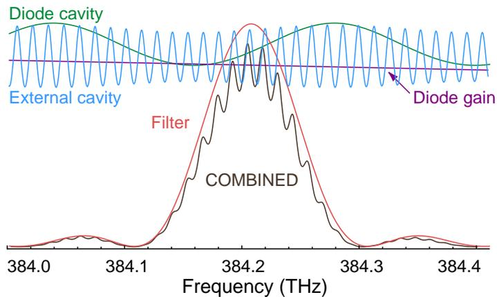
**Figure 3.2:** Schematic representation for the various frequency-dependent factors of an ECDL, adapted from Ref. [1], for wavelength  $\lambda = 780$  nm and external cavity length  $L_{\text{ext}} = 15$  mm.
