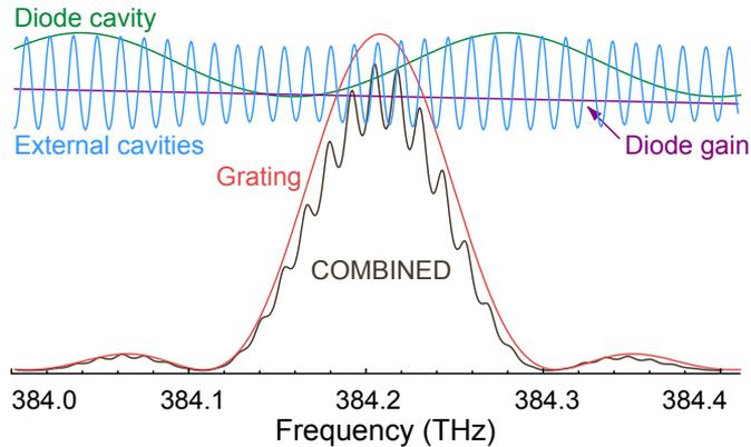
**Figure 1.4:** Schematic representation for the various frequency-dependent factors of an ECDL, adapted from Ref. [1], for wavelength  $\lambda = 780$  nm and external cavity length  $L_{\text{ext}} = 15$  mm.
