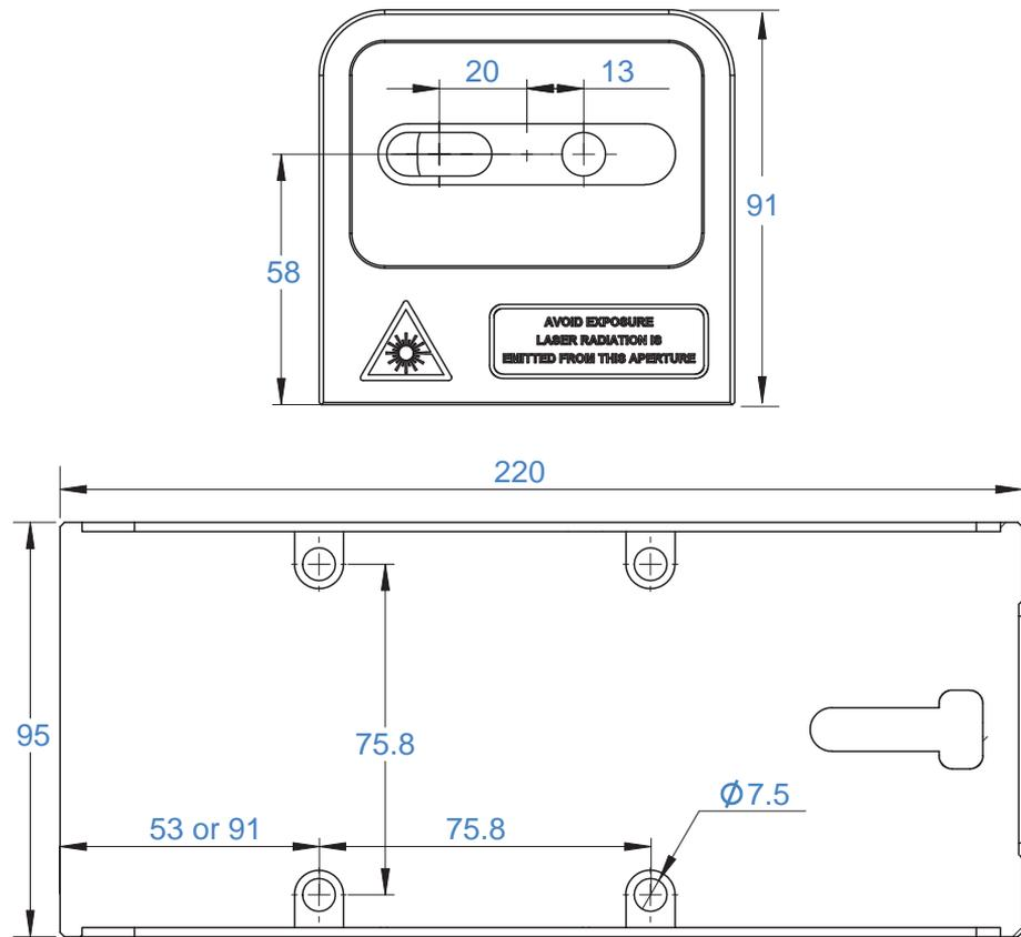
Figure A.3: Dimensions of CEF laser head.
