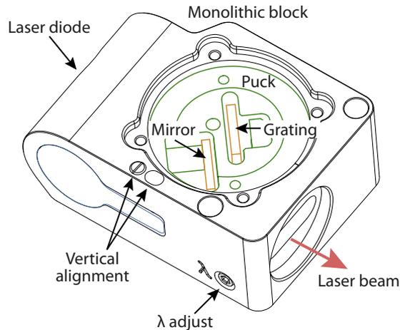
Figure 1.1: Sketch of MOGLabs LDL monolithic block external cavity diode laser.
