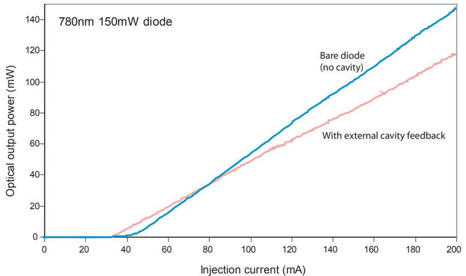
**Figure 2.1:** Sample laser diode power-current  $PI$  characteristic curves, with and without an external cavity. The external cavity feedback reduces the threshold current, and also the apparent power/current slope because the measured power with feedback is not the power from the bare diode, but the output beam reflected from the grating. The slope with feedback in this example is 75% of the bare diode output slope, consistent with the grating direct reflectivity.
