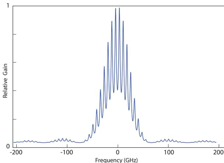
**Figure 3.3:** Combined gain for an external cavity diode laser, including the internal and external modes, the diode laser gain, and the filter response. The broad feature is the frequency selectivity of the filter, and the smaller peaks are the external cavity modes (see fig. 3.2). A small relative shift of the external cavity mode relative to the filter frequency will cause the laser to jump to another external cavity mode where the net gain is higher.
