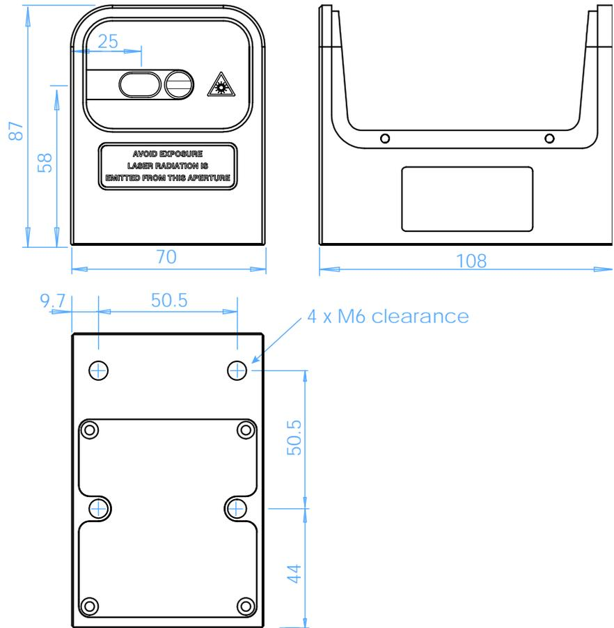
Figure A.1: Dimensions of compact LDL laser head.
