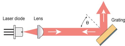
**Figure 1.2:** Schematic of a Littrow configuration external cavity diode laser (ECDL). The external cavity, formed by the rear facet of the laser diode and the grating, determines the laser wavelength. One longitudinal cavity mode is selected by dispersive feedback from the grating.
