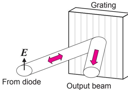
**Figure 4.3:** Orientation of the diode laser beam ellipse with respect to the diffraction grating.
